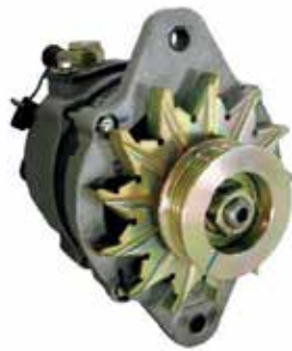
OE NO. 26021117 RGT 4041 ALT ALTERNATOR 12V 65A 35A23 TATA 207 TELCOLINE 1.9 DIESEL
