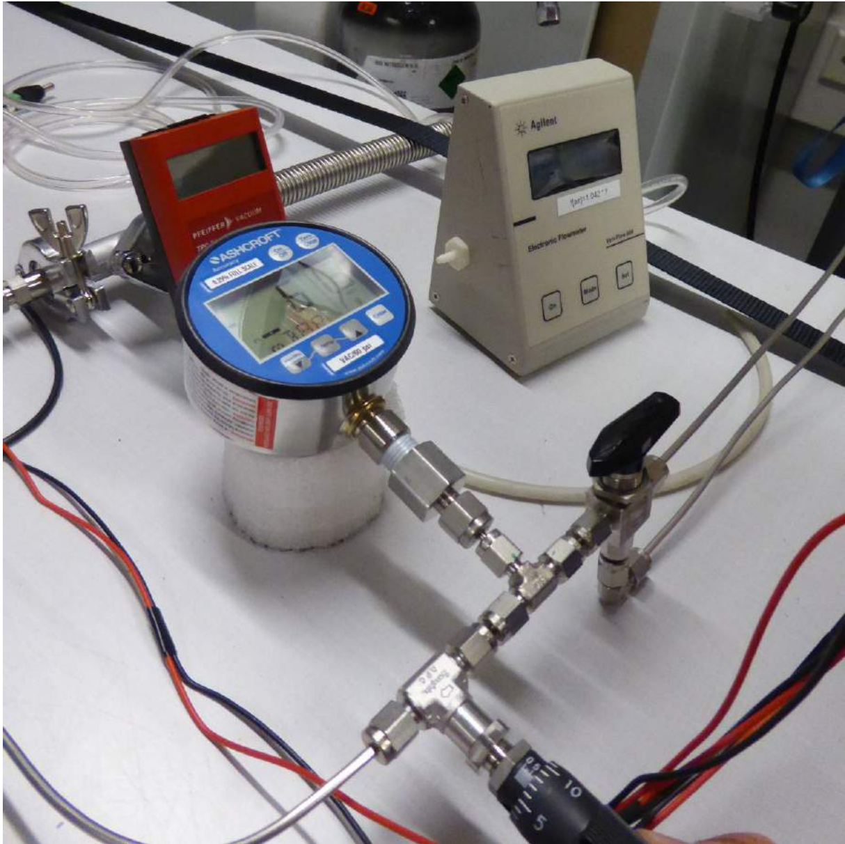
Figure 148: Valve that Controls Filling/Vacuum in of the Sampling Bags. Pressure Sensor, Flow-metre and Needle Valve.
