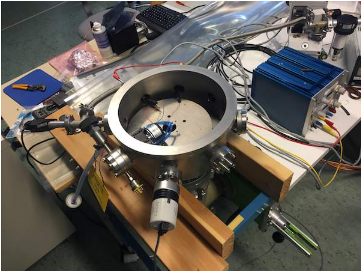
Figure 136: Photo Showing the Set-up of the Vacuum Chamber, Power Supply and Vacuum Pump.
