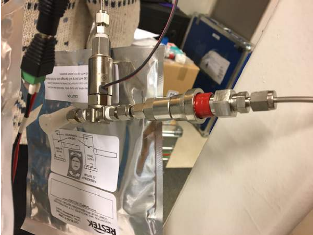
Figure 145: 1 L Sampling Bag With SMC Valve Attached to It. The Valve is at One of the Ends of the System so a Quick Connector is Connecting it to the Tube That Goes to the Nitrogen Bottle/Vacuum Pump.
