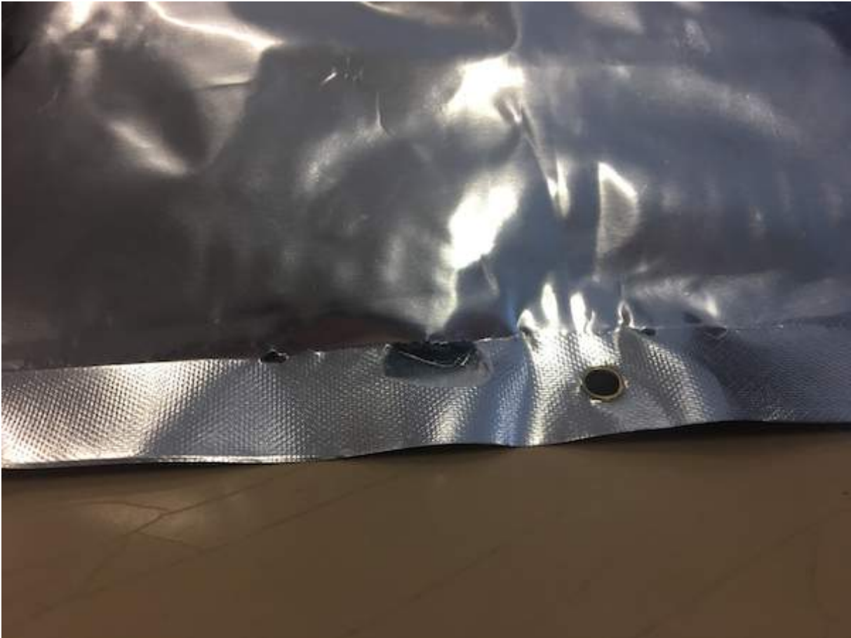
Figure 140: Photo Showing the Extent of Damage on the Back of the Bag Due to Bursting.
