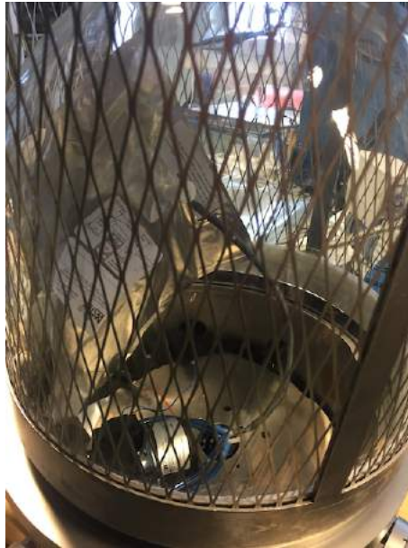
Figure 137: Photo Showing the Pump and Sampling Bag in the Vacuum Chamber During the Test.
