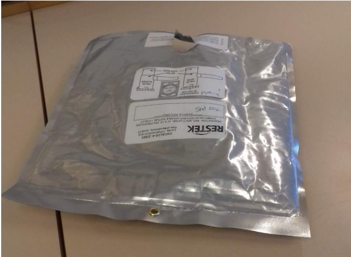
Figure 142: Photo Showing Where the Bag Ripped Around the Valve.
