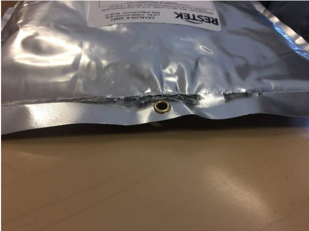
Figure 139: Photo Showing the Extent of Damage on the Front of the Bag Due to Bursting.
