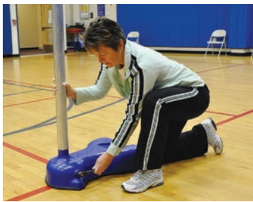
Slide down telescoping upright and roll to storage
