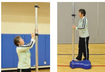
Slide down telescoping upright and roll to storage
