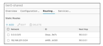
For each Tenant Tier-0 router, the default static route should point to the tenant's corporate network. As shown in the image below, the Tenant Tier-0 defines a static route to the corporate network as 0.0.0.0/0:
