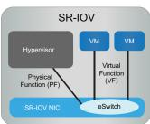
Network Function Virtualization (NFV), enabling a VM to be used as a virtual appliance. The full datapath operation offloads, hairpin hardware capability and service chaining enables data to be handled by the virtual appliance, with minimum CPU utilization.
