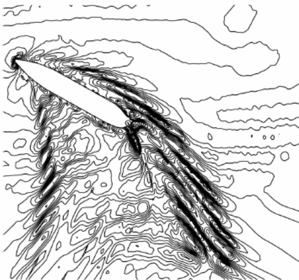
Figure 3.8- Free Surface Deformation during a Turning-Circle Manoeuvre of a Container Ship. \Psi=60^\circ (Jensen et al., 2004).
