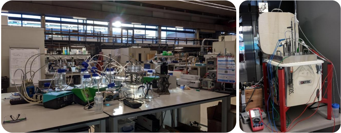
Figure 7-4 - The used experimental setup of the combination of ED, BPMED and VMS (left) and the SOFC (right).
