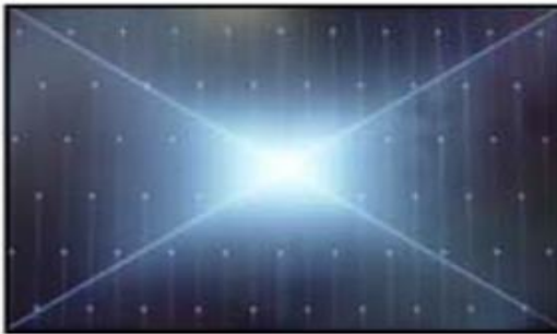
Solder defect, Short/Crack
