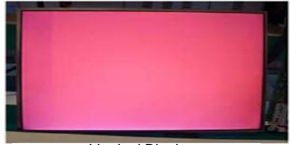
Vertical Block Source TAB IC Defect
