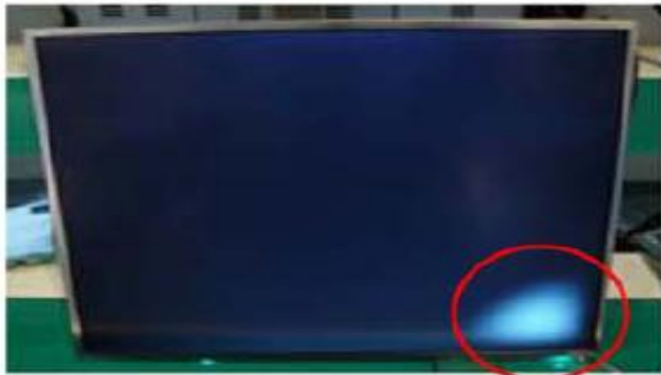
Panel Mura, Light leakage
