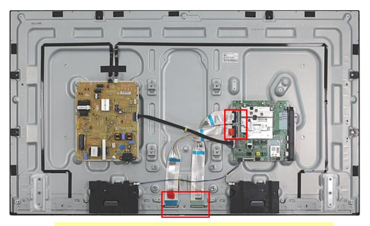
Check the contact condition of the Link Cable, especially dust or mis insertion.
