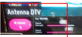
When the signal is strong, use the attenuator (-10dB, -15dB, -20dB etc.)
