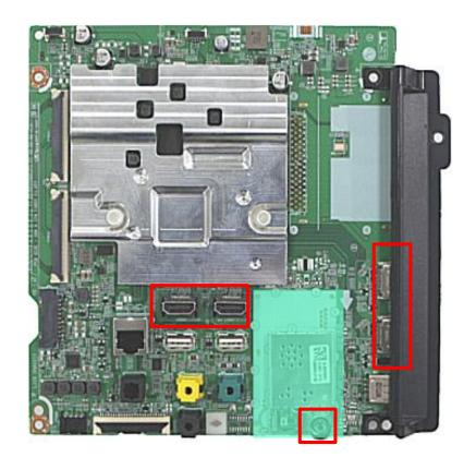
As the part connecting to the external input, check the screen condition by signal
