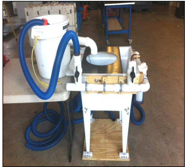
Figure B-3. Infauna sample sieving apparatus
