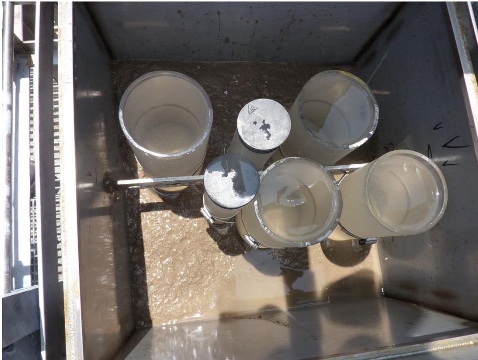
Figure 2. Box corer being deployed from the deck of Adriatic Marine M/V IRISH . (B) Interior view of box corer.
