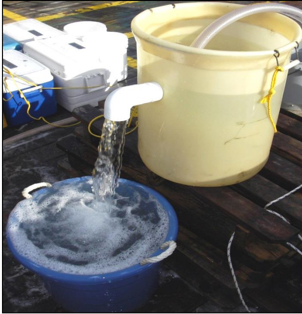
Figure B-2. Infauna sample sieving apparatus consisting of an upper holding barrel and lower spill over barrel.
