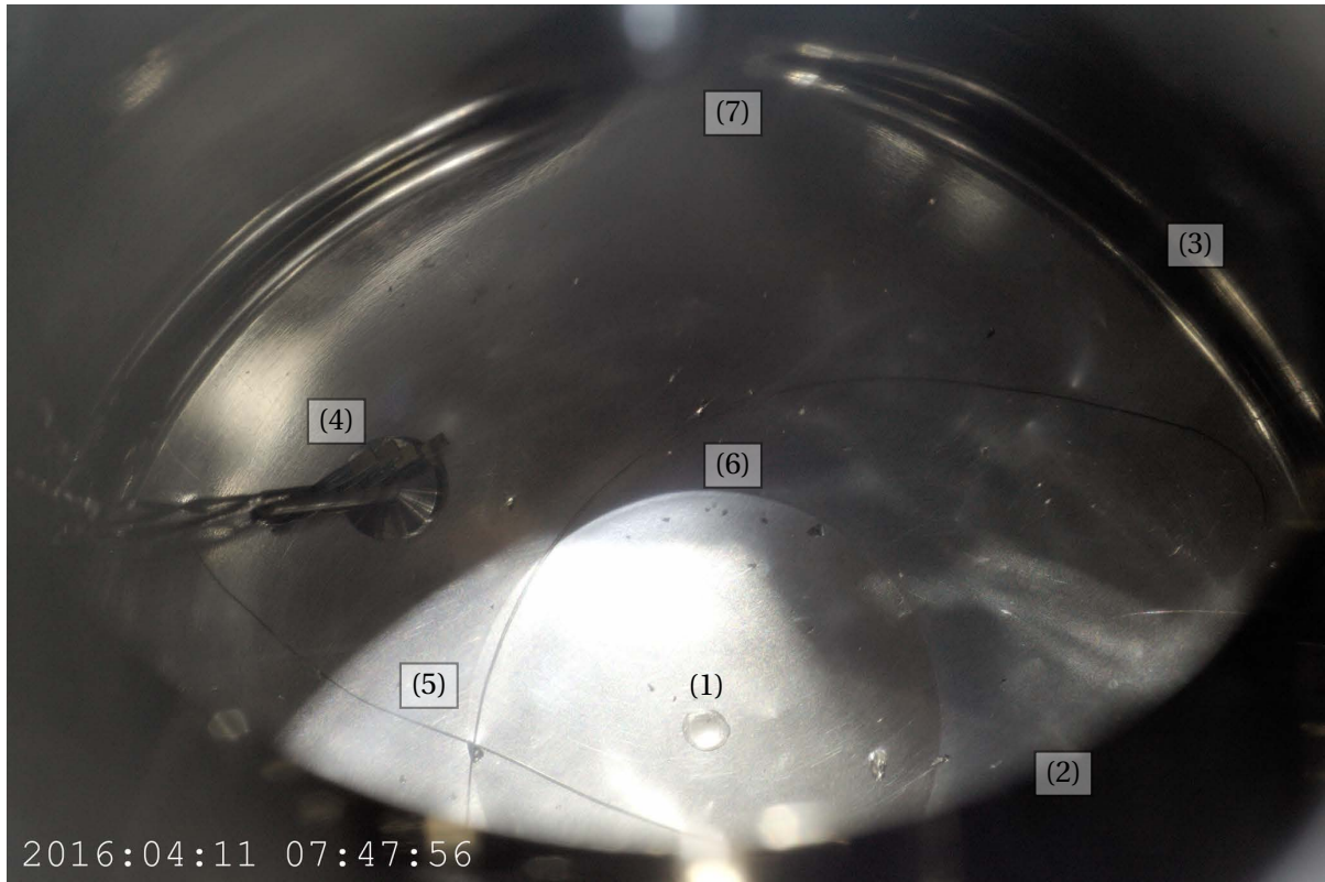
Figure 5.6: Photo of the empty deuterium container seen through the monitoring system. The view from above is shown in Figure 5.8. The residual deuterium in the cryostat has been condensed at center of the deuterium container, located below (1). This confirms that the center of the container is the coldest point. The lower arc at (2) is the bottom edge of the mirror. The upper arc at (3) is the edge of the container, a fillet where the bottom meets the vertical walls. (4) is the embedded temperature sensor holder. Unfortunately, there is evidence of issues with the neutron guides. The crossing lines at (5) are titanium wires used to support the lowest neutron guide. They should be located above the deuterium container, and out of the focal plane of the image, and so have evidently broken free and are lying on the bottom of the container. The container has a mirror finish, and the many specks seen, for example at (6), are most likely pieces of nickel coating fallen from the guides above. The distortion at (7) is caused by the screws used to mount the mirror.
