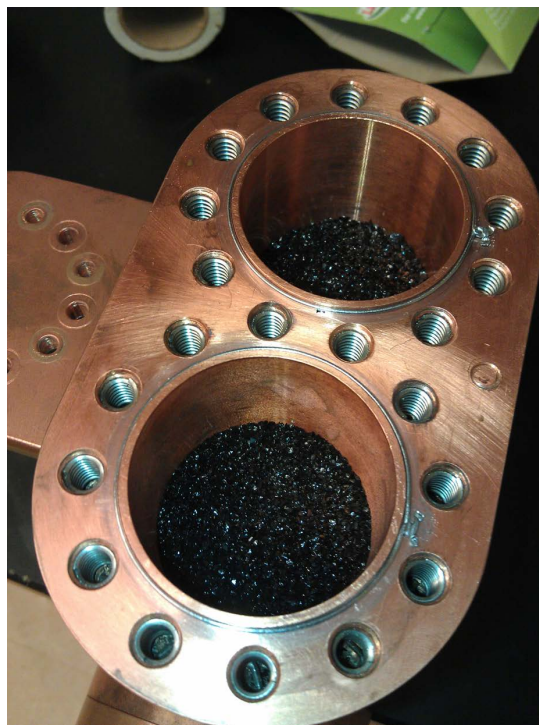
Figure 4.29: The converter cell filled with roughly 350 mL iron hydroxide.
