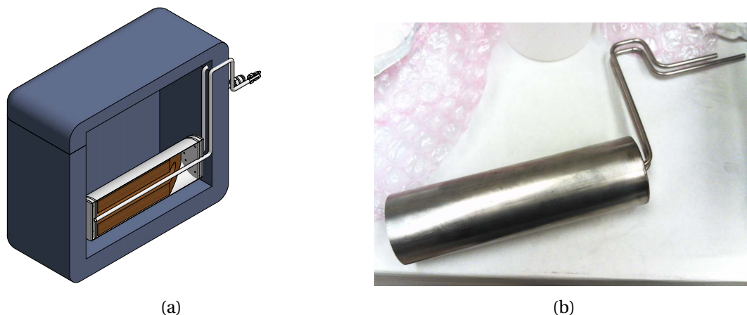
Figure 4.13: (a) A CAD cross-section of the liquid nitrogen gas trap and styrofoam container and (b) a photo during assembly.
