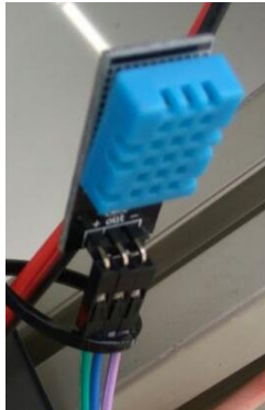
Gambar 3.22 Sensor suhu DHT11
