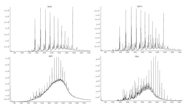
**Figure 3.** Chromatograms of four different sites (ROD, JQT, ARN and TRA) analyzed by gas chromatography coupled to flame ionization detection (GC-FID).
