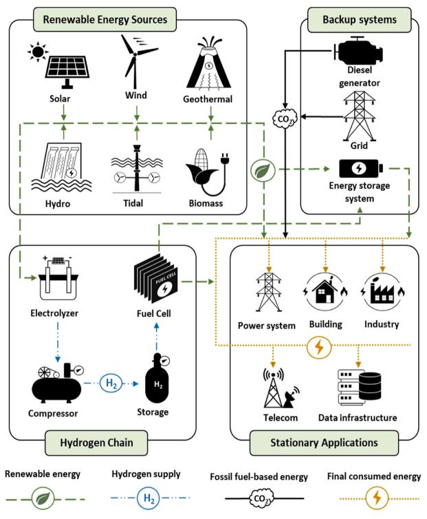
Fig. 2. RHS power supply chain for stationary applications.
