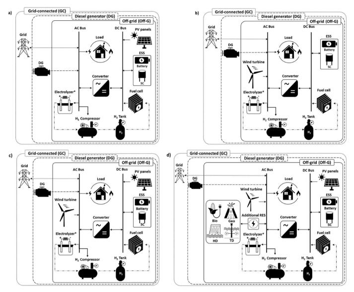
Fig. 3. Binary PV/FC (a), binary WT/FC (b), ternary PV/WT/FC (c), and multi-generation RHS (d). \* Electrolyzer includes AC/DC rectifier.
