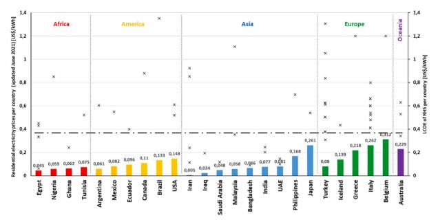
Fig. 4. Comparison between residential electricity prices and LCOE of renewable hydrogen-based schemes analyzed per country. Dotted and dashed line represents the maximum reported residential electricity price (0.365 US\$/kWh) in Germany.
