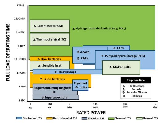
Fig. 1. Operating parameters of different energy storage systems. Abbreviations: ACAES (Adiabatic Compressed Air Energy Storage), CAES (Compressed Air Energy Storage), LAES (Liquid Air Energy Storage). Adapted from Ref. [71].
