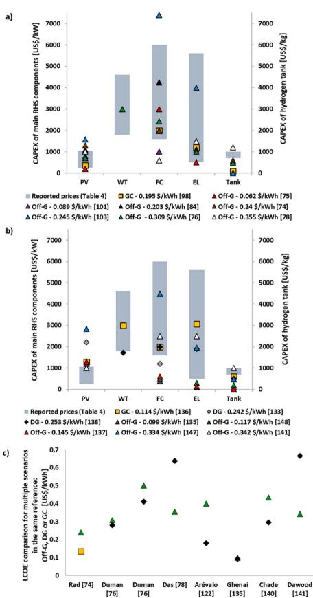
Fig. 5. CAPEX comparison of small-medium scale (a) and large-scale (b) RHS with competitive LCOE. (c) LCOE comparison in multiple scenarios in the same reference (triangles are employed for components costs from Off-G configurations, squares for GC systems, and diamonds for DG).
