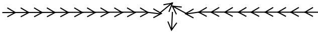
Fig. 4. Distribution of magnetic dipole moments in the absence of an external field.
