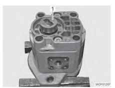
Fig. 153 Gear pump housing
