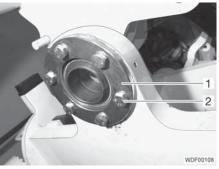
Fig. 292 Securing the lower bearing
