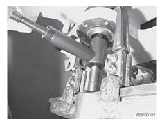
Fig. 291 Removing the shaft
