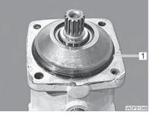
Fig. 121 Sealing the variable displacement motor
