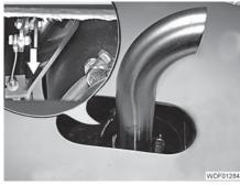
Fig. 280 Locking mechanism of engine hood
