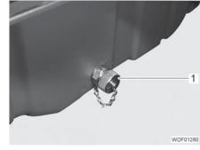
Fig. 33 Oil drainage screw
