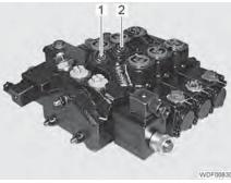
Fig. 32 Test connection
