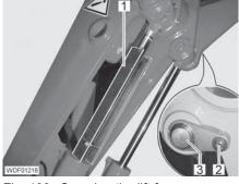
Fig. 193 Securing the lift frame
