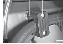
Fig. 74 Hydraulic line attachment
