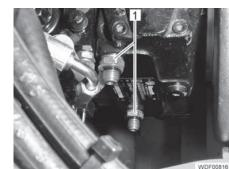
Fig. 16 Screw attachments
