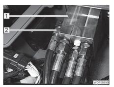
Fig. 354 Front attachment of the Bowden cable
