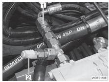
Fig. 29 Test connection P<sub>H</sub>
