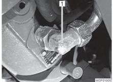
Fig. 259 Hydraulic line of the cross flushing connection
