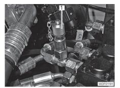
Fig. 37 Test connection
