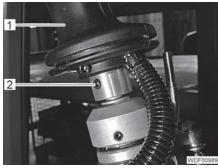
Fig. 209 Multi-function lever attachment
