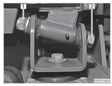
Fig. 343 Cab attachment (front)
