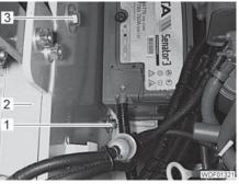
Fig. 95 Drainage screw
