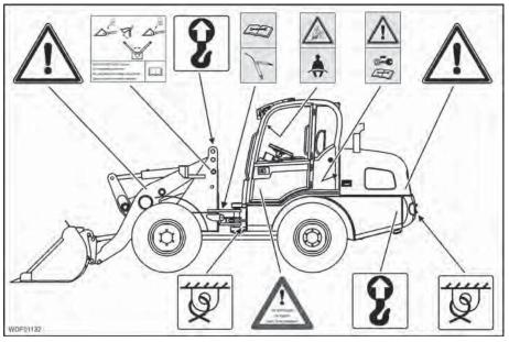
Fig. 1 Stickers located on the left in the driving direction
