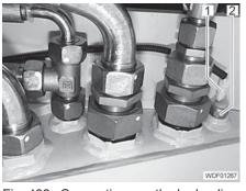
Fig. 433 Connections on the hydraulic fluid tank
