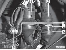
Fig. 335 Main brake cylinder
