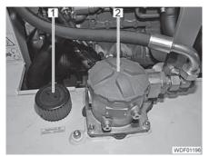
Fig. 101 Depressurizing the hydraulic system
