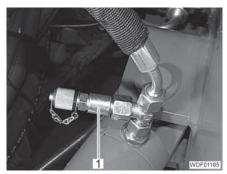
Fig. 24 Test connection
