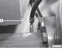
Fig. 235 Hydraulic line of the differential lock
