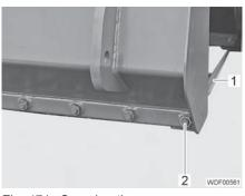
Fig. 471 Securing the prong
