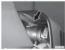
Fig. 89 Position of the air filter
