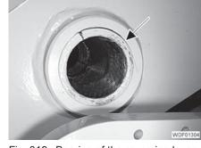
Fig. 319 Bearing of the reversing lever
