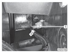
Fig. 275 Cable for the rear lighting (alternative)
