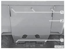
Fig. 273 Base plate attachment
