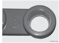
Fig. 302 Underside of the self-aligning bearing
