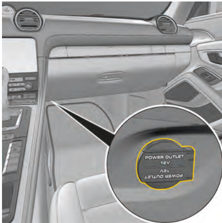
Fig. 169: Electrical socket in footwell
