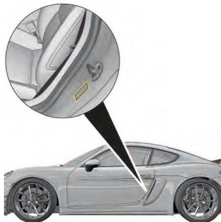
Fig. 186: Tire pressure plate on door sill
