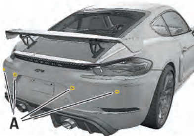
Fig. 99: Ultrasound sensors for distance measurement
