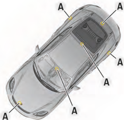
Fig. 50: Installation position of the radio antennas
