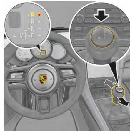
Fig. 86: Switching gear lever position
