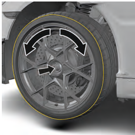
Fig. 204: Place the wheel on the wheel hub
