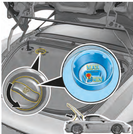
Fig. 179: Coolant reservoir 718 Spyder RS
