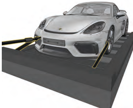
Fig. 177: Tie vehicle down on flatbed
