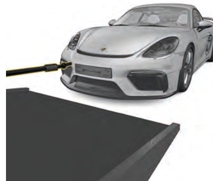
Fig. 176: Pulling the vehicle onto the flatbed
