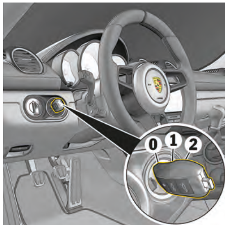
Fig. 83: Ignition lock settings
