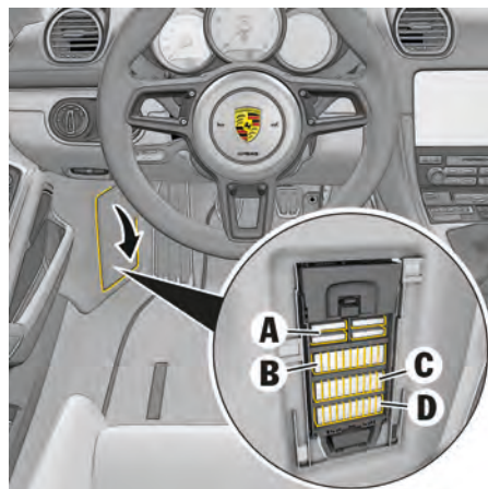
Fig. 217: Fuse carrier in driver's side footwell
