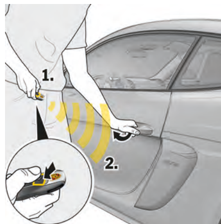
Fig. 46: Unlocking doors with the vehicle key
