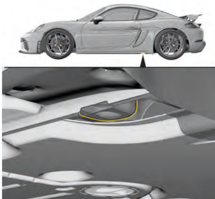
Fig. 220: Rear jacking point for lifting platform or jack
