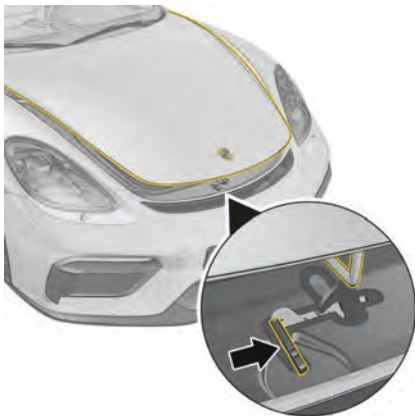
Fig. 10: Unlocking the front luggage compartment lid
