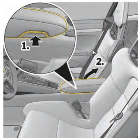
Fig. 153: Opening storage compartment in armrest on center console
