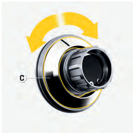
Fig. 201: Check the conical ring
