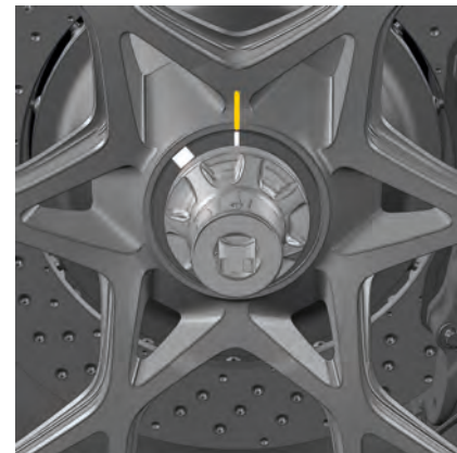
Fig. 214: Markings on the central bolt
