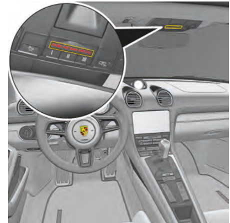
Fig. 51: PASS AIR BAG OFF/ON indicator
