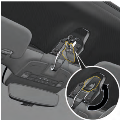
Fig. 33: Locking convertible top latch
