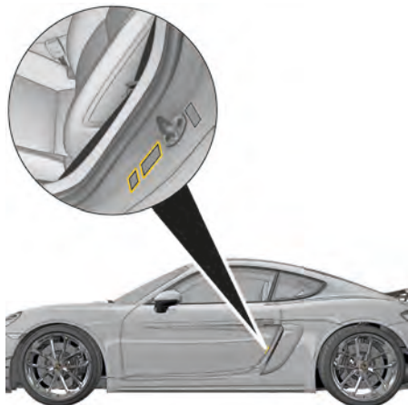
Fig. 224: Location of tire pressure plate
