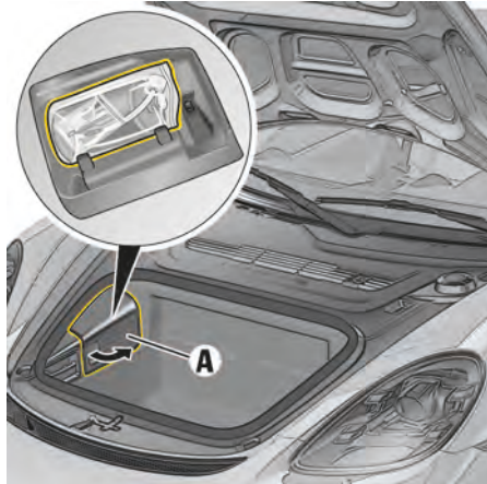
Fig. 159: Plastic box A with tire sealant (Tire Mobility System – TMS)
