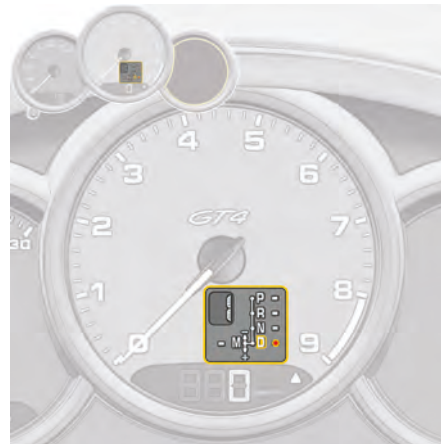
Fig. 87: Gear lever position and engaged gear display
