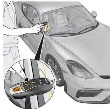
Fig. 47: Emergency unlocking with faulty remote control
