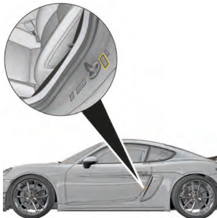
Fig. 223: Placement position of safety conformity stickers
