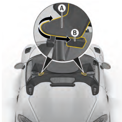
Fig. 41: Removing convertible top fins from bracket
