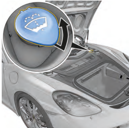
Fig. 221: Washer fluid reservoir for windshield and headlights
