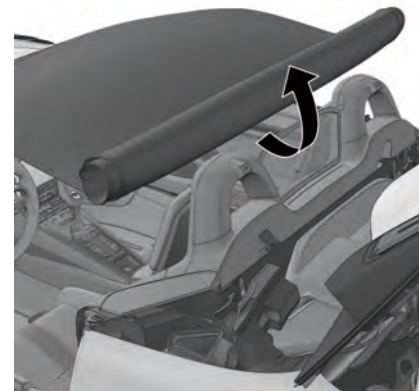
Fig. 26: Rolling up convertible top
