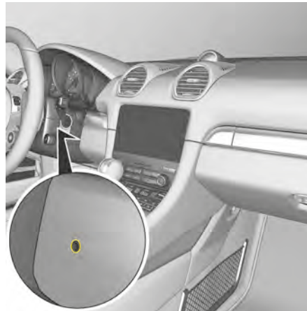
Fig. 58: Interior temperature sensor
