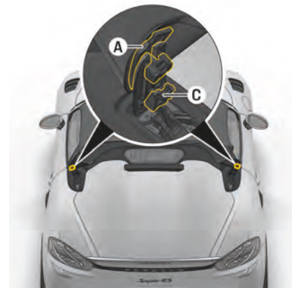
Fig. 43: Inserting and tensioning convertible top fins
