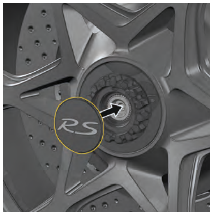
Fig. 210: Mount the cap
