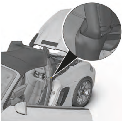
Fig. 40: Checking rubber seal for correct seating
