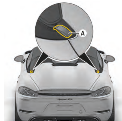
Fig. 17: Pull release tabs
