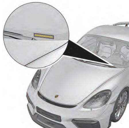
Fig. 222: Location of vehicle identification number
