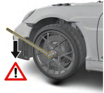
Fig. 200: Removing the central bolt
