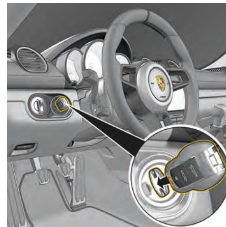
Fig. 82: Inserting the vehicle key in the ignition lock
