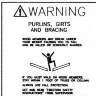
Wood Member Warning
