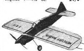
VIPER. Tough 27½" span stunt trainer with profile fuselage for engines 1—1.5 cc. 24/6
