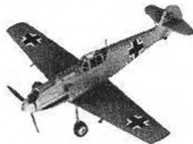
ME 109. Scale model of all balsa construction for engines of 1.5 cc. Span 21". 41/11
