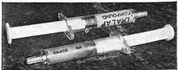
Above, lapping the bore using the special tool. Below, Five Pounds worth of diamond abrasive (2 grams. in each syringe).
