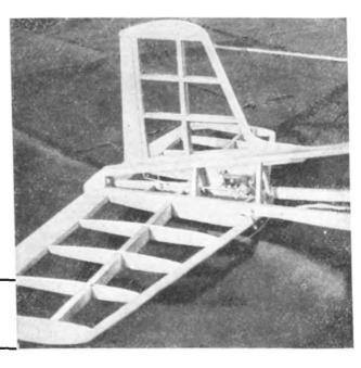
The constructional photographs on this and previous pages, together with the cut-away drawing, give an indication of the simple yet efficient design of this outstanding model. Close-up of tail unit shows installation of the magnetic actuator (Pros. Patent No. 29978) used on the "Aeromodeller" Rudder Bug, brain child of cur old friend Howard Boys.
