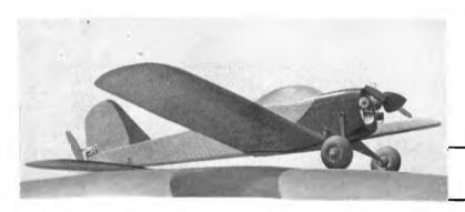
Heading photo :—Control-line Boeing P-12F built in Kansas. Power is a Vivell 35 petrol motor. On left :—Low-wing R/C model by Dick Schumacher of Resedo, California.
