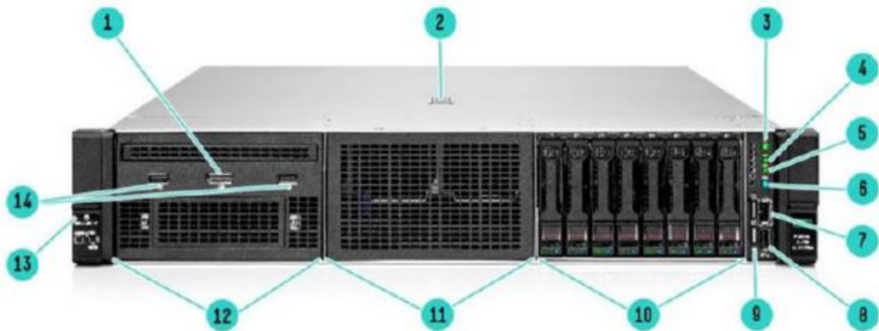
Front View - SFF chassis with optional Universal Media bay shown
