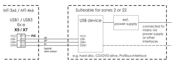
Type 2 connection diagram (e.g. hard disk, CD/DVD with power supply)
