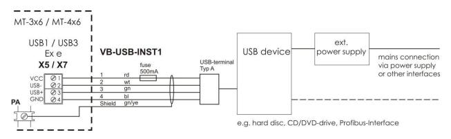
Connection diagram with VB-USB-INST1 (hard disk, CD/DVD with power supply)
