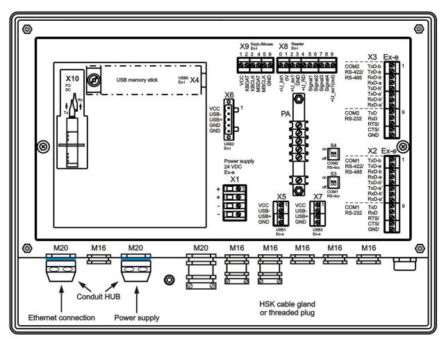
Any cable glands at the operator interface that are not required **<u>MUST BE</u>** replaced by threaded plugs so that the opening in the housing is covered.
