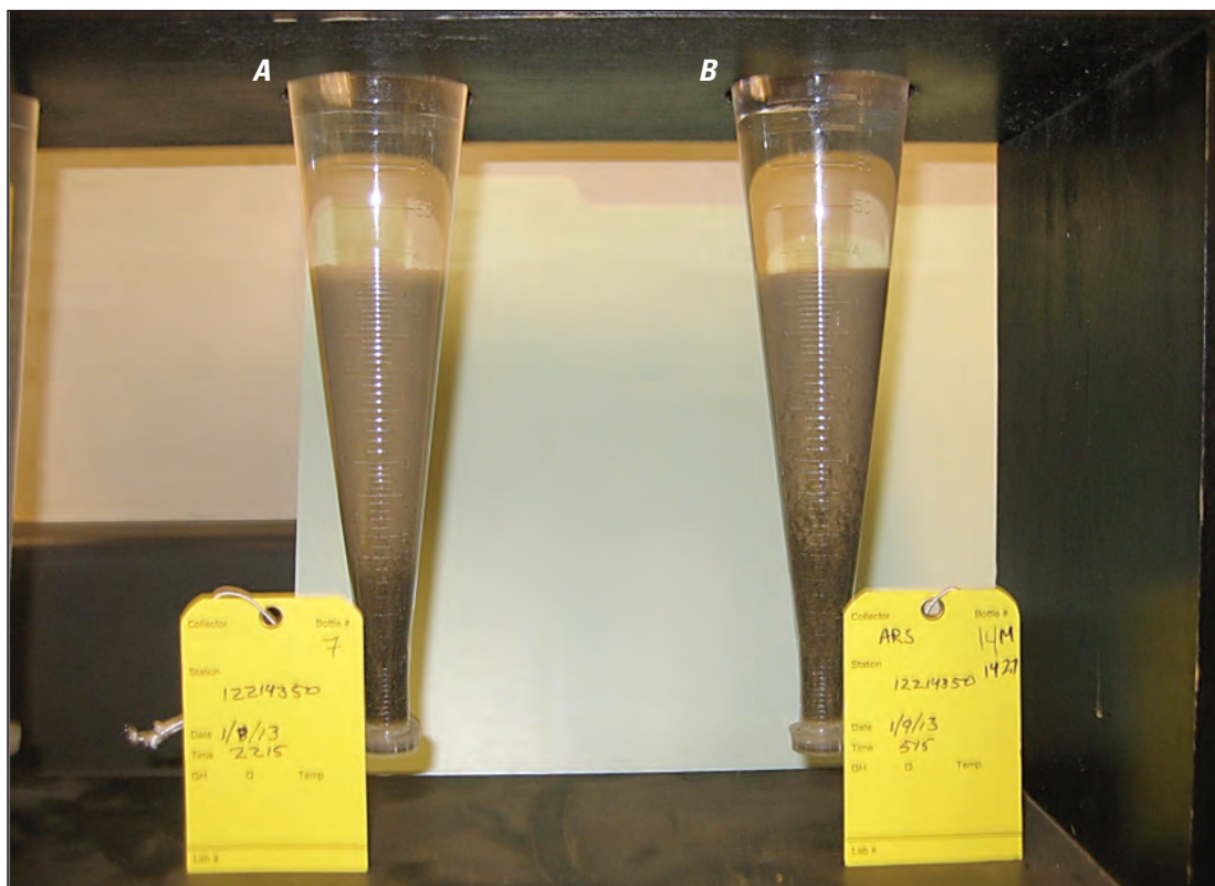
Figure 15. Two samples of suspended sediment collected from Sumas River at South Pass Road at Nooksack (12213500), Washington during a winter storm on January 8 and 9, 2013. Samples were allowed to settle in a 1-liter Imhoff cone. Sample A collected on January 8 at 2215 shown on the left; sample B collected on January 9 at 0515 shown on the right.
