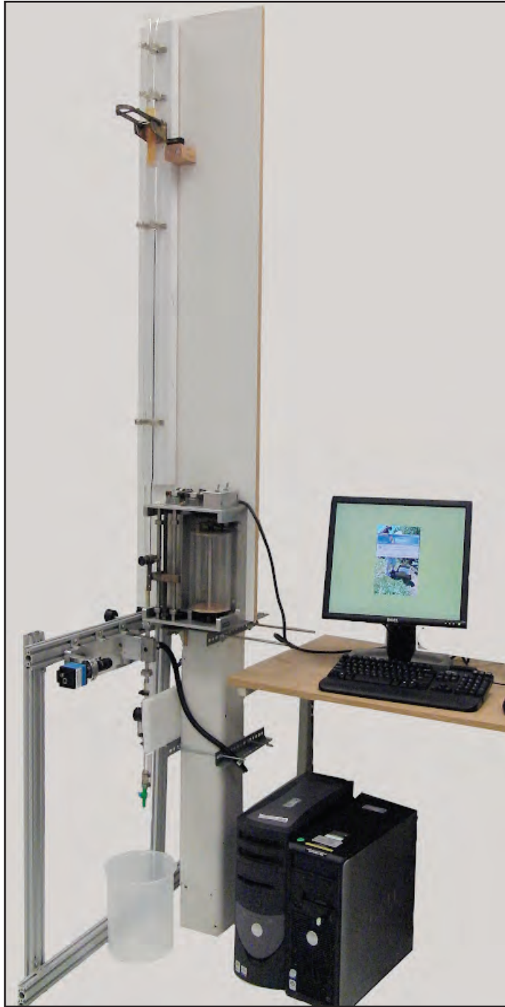
Figure 22. Laboratory apparatus used to measure the settling velocity of sediment samples collected from the Sumas River, Whatcom County, Washington. Measurements were done at the U.S. Geological Survey sediment laboratory at the Cascade Volcano Observatory, Vancouver, Washington.
