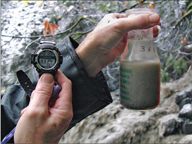
Figure 4. Sediment sample collected from Swift Creek near the toe of the Swift Creek landslide, Whatcom County, Washington. Note the distinct interface between the upper phase of clearer water and the flocculated phase that settles with time. Photograph by Christopher Magirl, U.S. Geological Survey, October 31, 2012.
