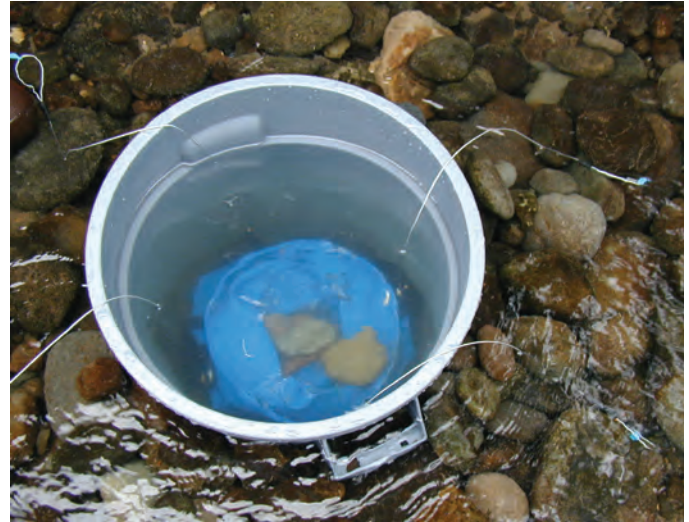
C. Collapsed bag with retrieval cables extending to the streambed surface
