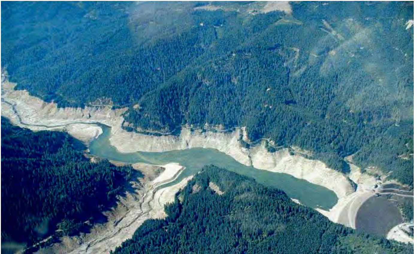
Figure 2. Aerial view of Cougar Reservoir during drawdown, with exposed upstream deltaic sediments, during the summer of 2002. (Photograph taken by U.S. Army Corps of Engineers, Portland District, Oregon, 2002.)
