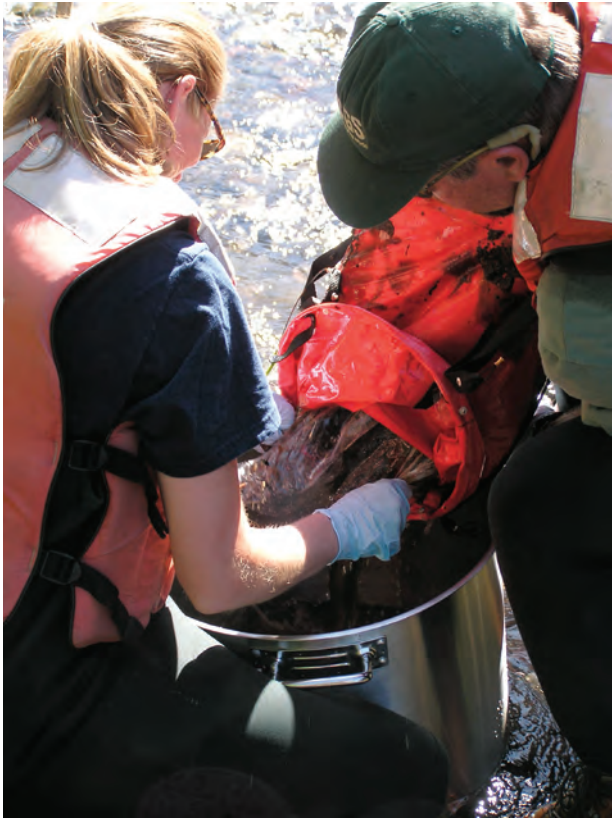
D. Pouring contents of the retrieved bag into a stainless steel bucket for subsampling
