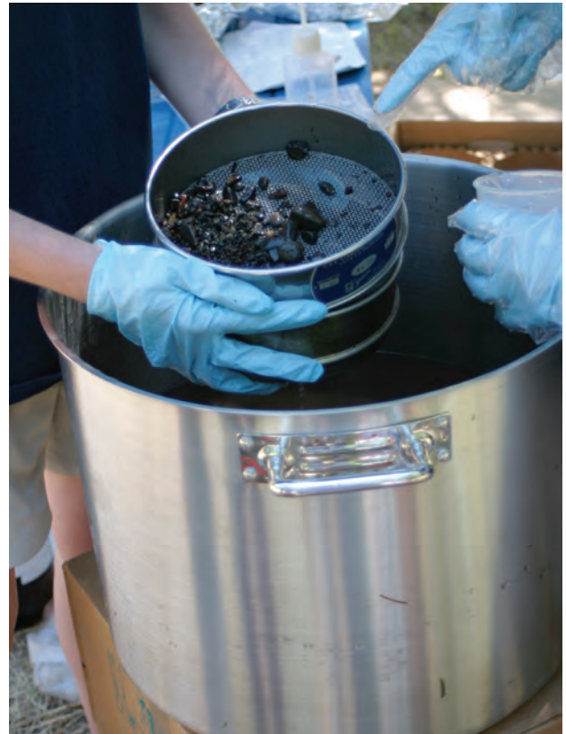
F. Sieving the remaining gravel to remove sand and larger sediments for size analysis
