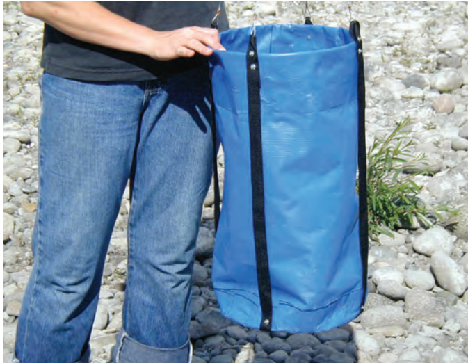
A. Constructed infiltration bag
