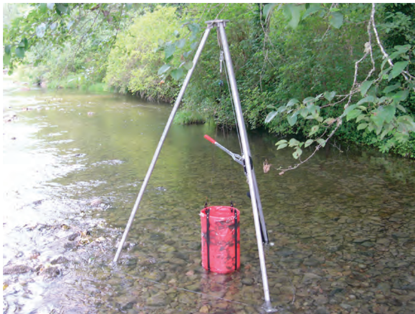
C. Tripod and winch retrieval system with a completely extracted infiltration bag
