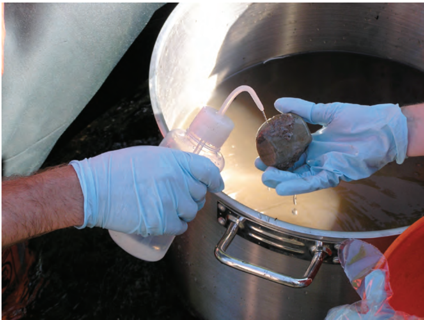
E. Washing individual rocks to remove fine sediment into the bucket
