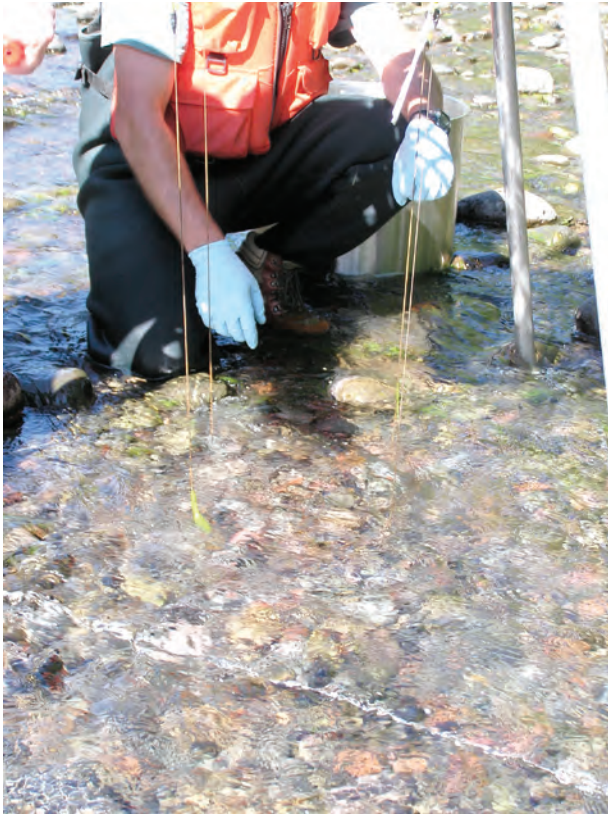
A. Tightened retrieval cables, with slight deformation of bed surface evident
