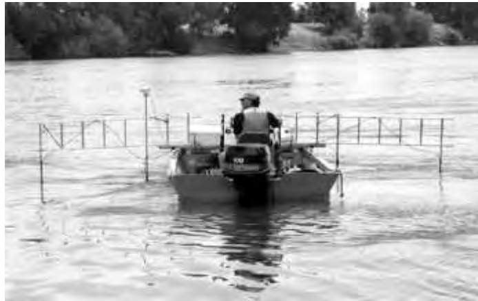
Figure 1. A small boat fitted with framework to suspend multiple sonar transducers and acquire depths and differential GPS data simultaneously.
