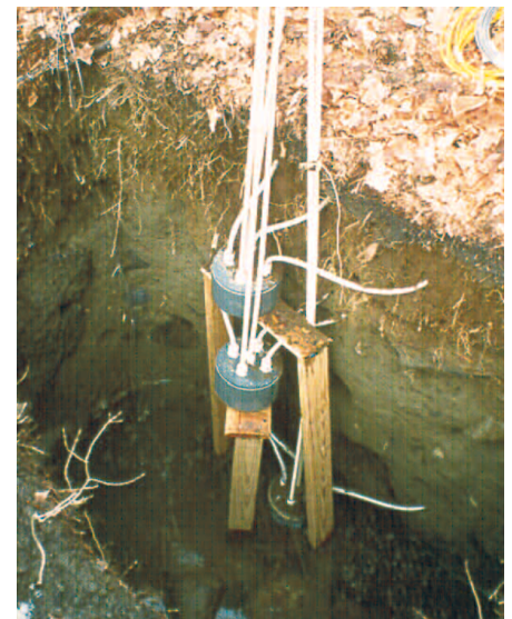
Permeable brown soil rich in fine roots overlies the dense olive-gray glacial till. The tubing and collection vessels are part of devices that collect water from the unsaturated zone of the soil.
