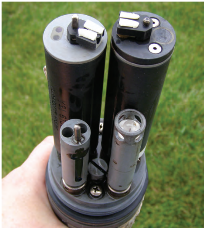
Figure 5. Continuous water-quality monitor with (clockwise from upper left) turbidity, optical dissolved oxygen, pH, and combined specific conductance and water temperature sensors.
