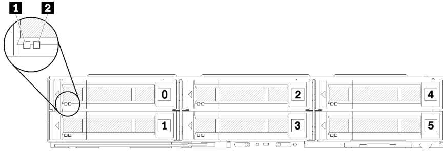
Figure 18. Six 2.5-inch drive configuration and drive bay numbering
