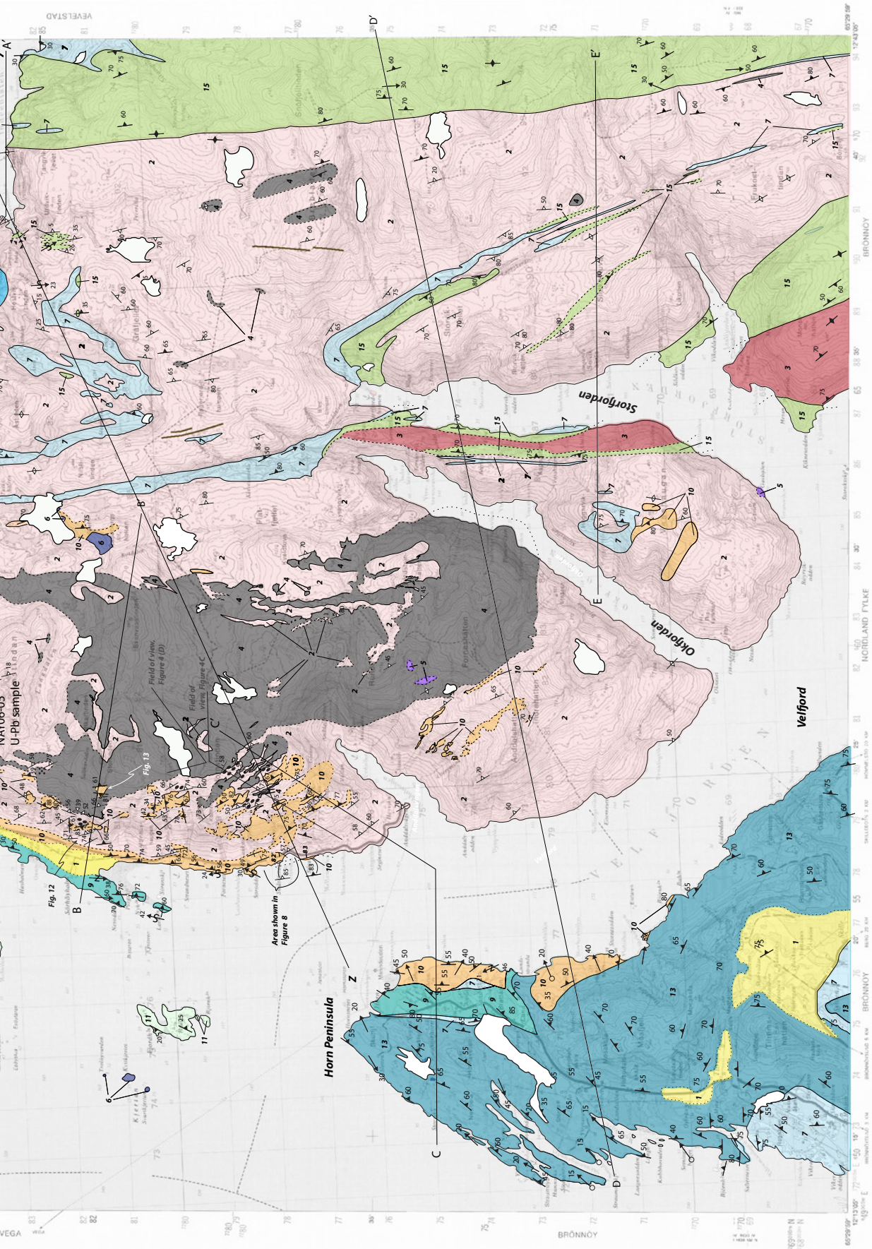
Figure 2. Geologic map of the Andalsshatten batholith. Geodetic datum: WGS84, UTM Grid, Zone 33, base map Vevelstad 1:50,000, Kartblad 1826 III. Base geologic map is from Nordgulen et al. (1992). Cross-section lines A-A', B-B', C-C', D-D', and E-E' are in Figure 3. Cross-section line z-z' is in Figure 14.
