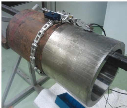
Figure 1. Phased array ultrasonic examination of the open piping test block.
