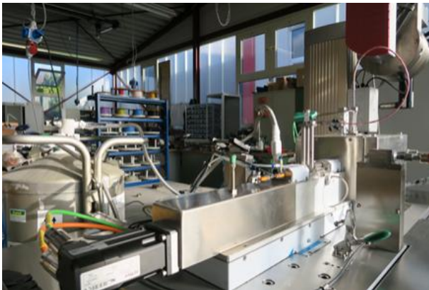
(above) Zwick HIT50 small impact tester with semi-automatic, remotely operated specimen furnace and feeder.
