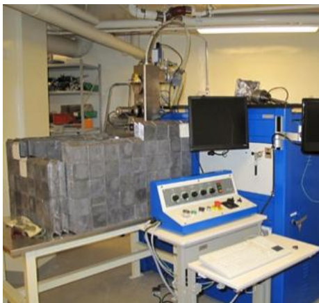
Figure 15: VTT’s electron beam welder (left) will be modified for integration into the new hot cell (right).
