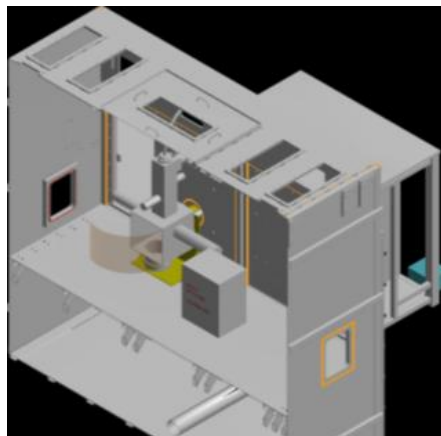
Figure 15: VTT’s electron beam welder (left) will be modified for integration into the new hot cell (right).
