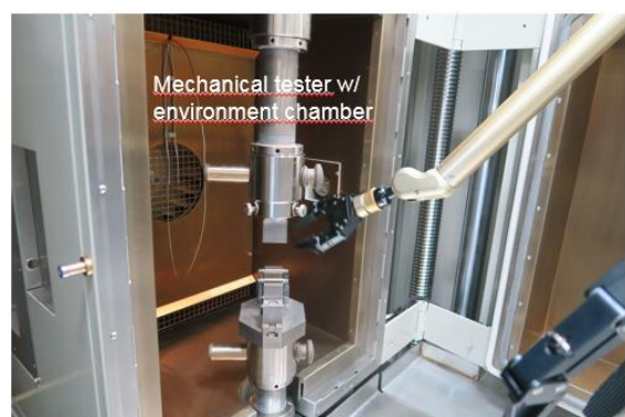
Figure 7: Factor acceptance tests of the two Zwick mechanical testing devices as they were integrated into the hot cells took place at ITD's factory.
