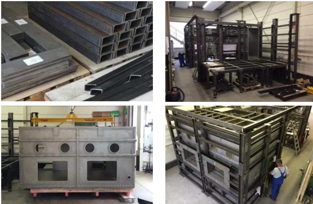
Figure 4: The hot cells are constructed from steel beams bolted together to make a frame that will support lead shielding bricks, and a stainless steel containment within which the radioactive materials are handled.
