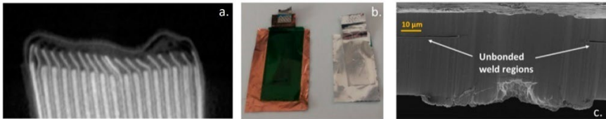
Figure 3.7: a) X-ray CT scan of electrode deformation in the prismatic cell; b) missing insulating tape on the cathode tabs; c) SEM cross-section of an anode tab weld (CC BY Loveridge et al. [104]).
