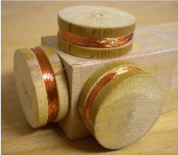
Figure16: The orthogonal coils at one end of the coil support.
