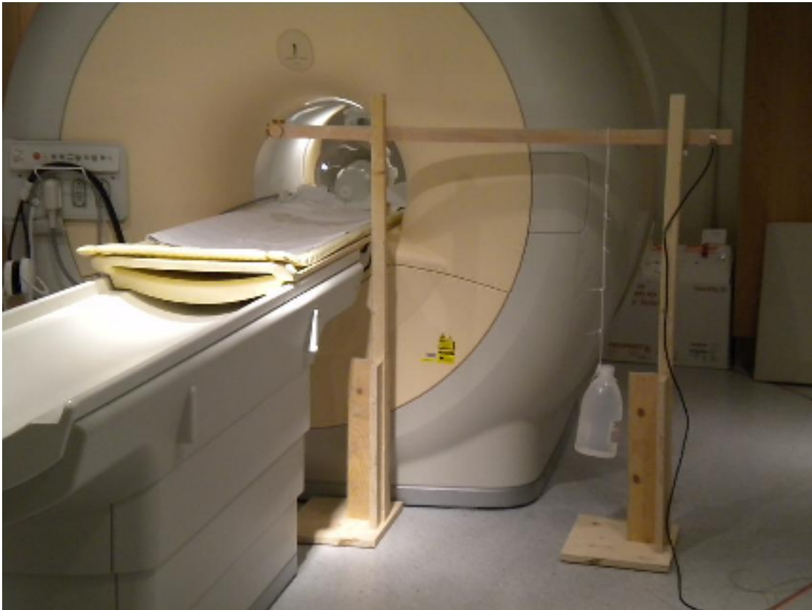
Figure 15: The stands, the coil support with the coils and a stabilizing weight mounted in front of the scanner.
