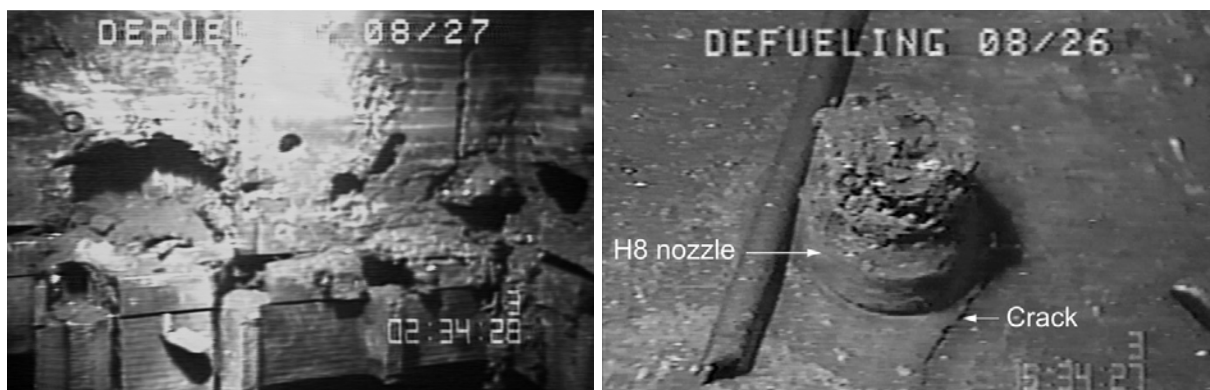
Figure 2. TMI-2 video examinations revealed locations where damage to core barrel and nozzles was more severe. (Courtesy of FirstEnergy)
