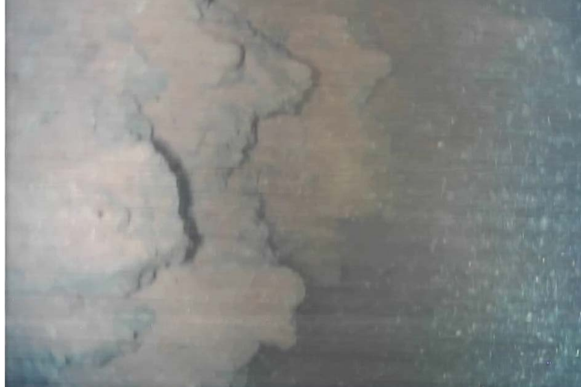
Figure 60. Image of material that had relocated beneath the 1F3 platform into the pedestal area; obtained on July 22, 2017 (Courtesy of TEPCO Holdings [211]).
