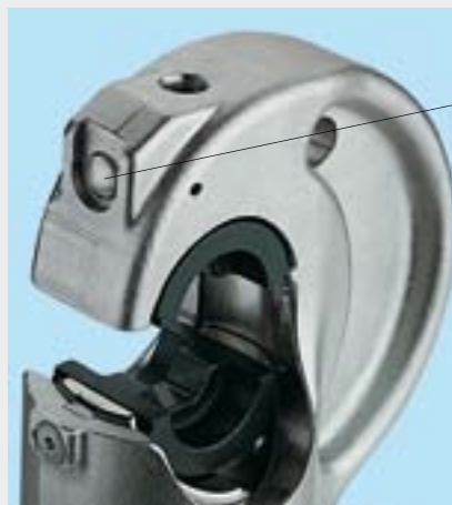
Die release system, protected from accidental operation
