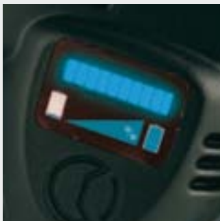
Battery condition display
