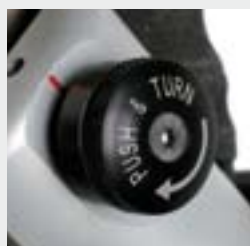
Detail of the pin for the quick jaws change
