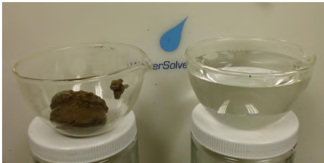
A one thousand milliliter sample conditioned with Solve 161 was poured through the GT500D Geotube® fabric. The captured cake (Left) and filtrate (Right) are shown above.
