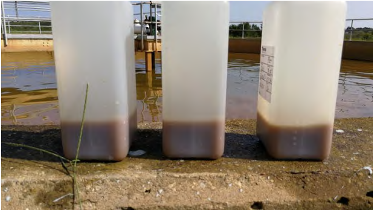
Photo 5: Sludge Samples after approximately 20-minutes of settling.
