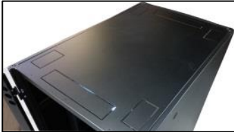
Top plate with unique cable entry Knock out holes with brushes, in front and rear. Over each 19" profile there is a unique hole which ensure that cables do not need to be bended more than necessary.
