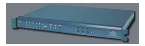
Etherstack's Off-Air-Monitors are non-intrusive intercept tools for trunked and conventional air interface testing and interoperability verification, maintenance and diagnostics.
