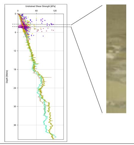
**Caption**: Shear strength variation between 2m and 6m attributed to the differing properties of constituent clasts in the debris flow deposit. (Note geohazard core only ~40cm length).
