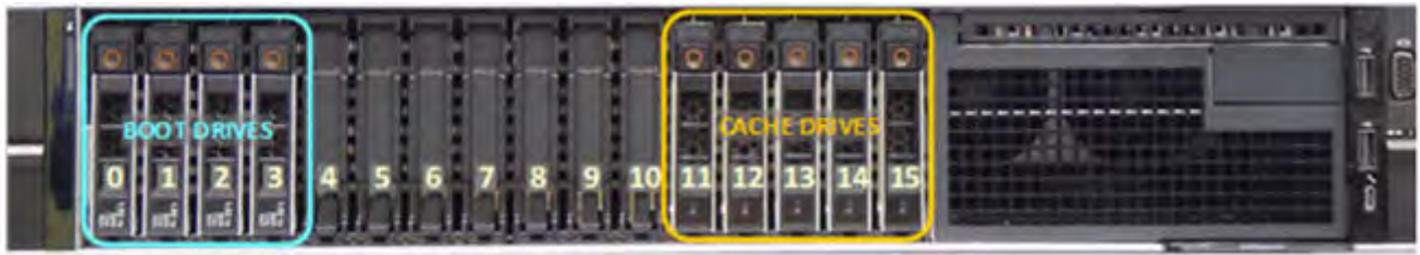
Figure 120. DD9400 SSD slot assignment (single node configuration)
