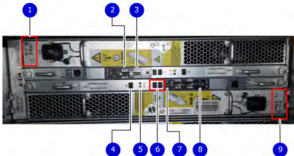
Figure 175. Back panel: Power modules and controllers
