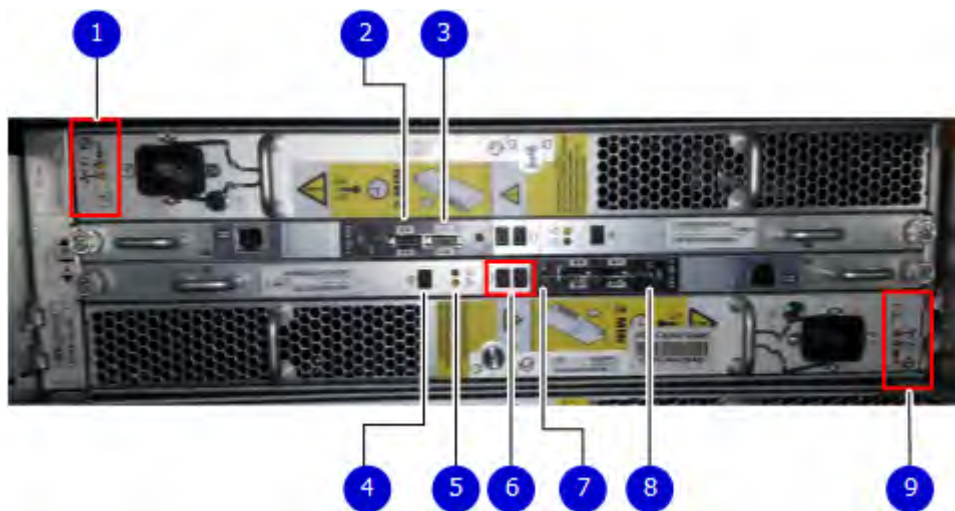
Figure 171. Back panel: Power modules and controllers
