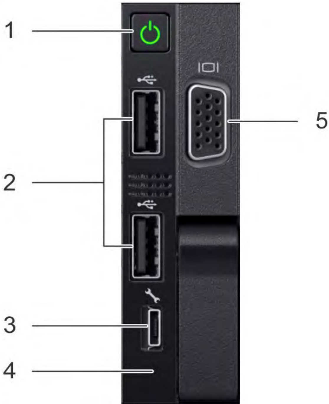
Figure 3. Right control panel
