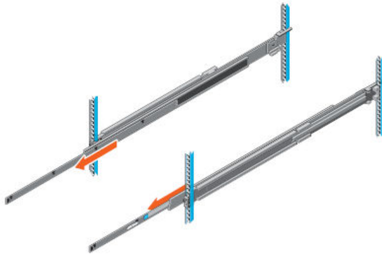
Figure 17. Pull the inner rails out of the cabinet
