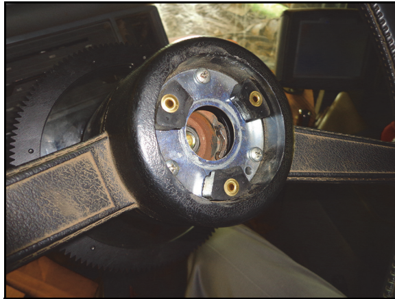
FIGURE 17. Steering Wheel Retainer Ring Reinstalled
