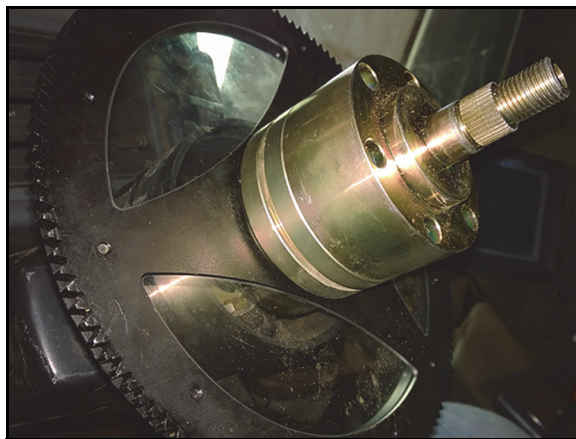
FIGURE 14. Spacers and Male Spline Installed
