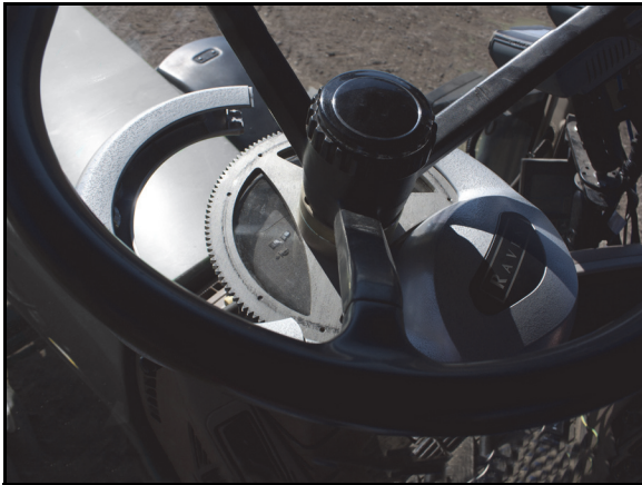
FIGURE 21. Mechanical Drive Installed
