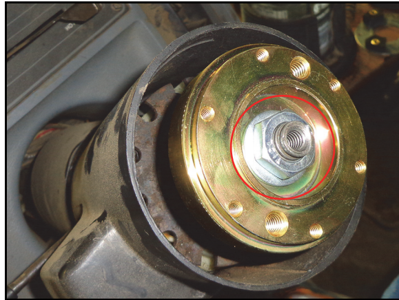
FIGURE 11. Steering Wheel Nut Installed
