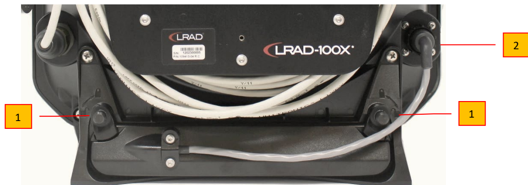
Figure 2 – LRAD-100X Battery Compartment
