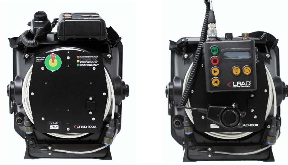
Figure 11 – Accessory Mounting: Top Option (left) and Rear Option (right)
