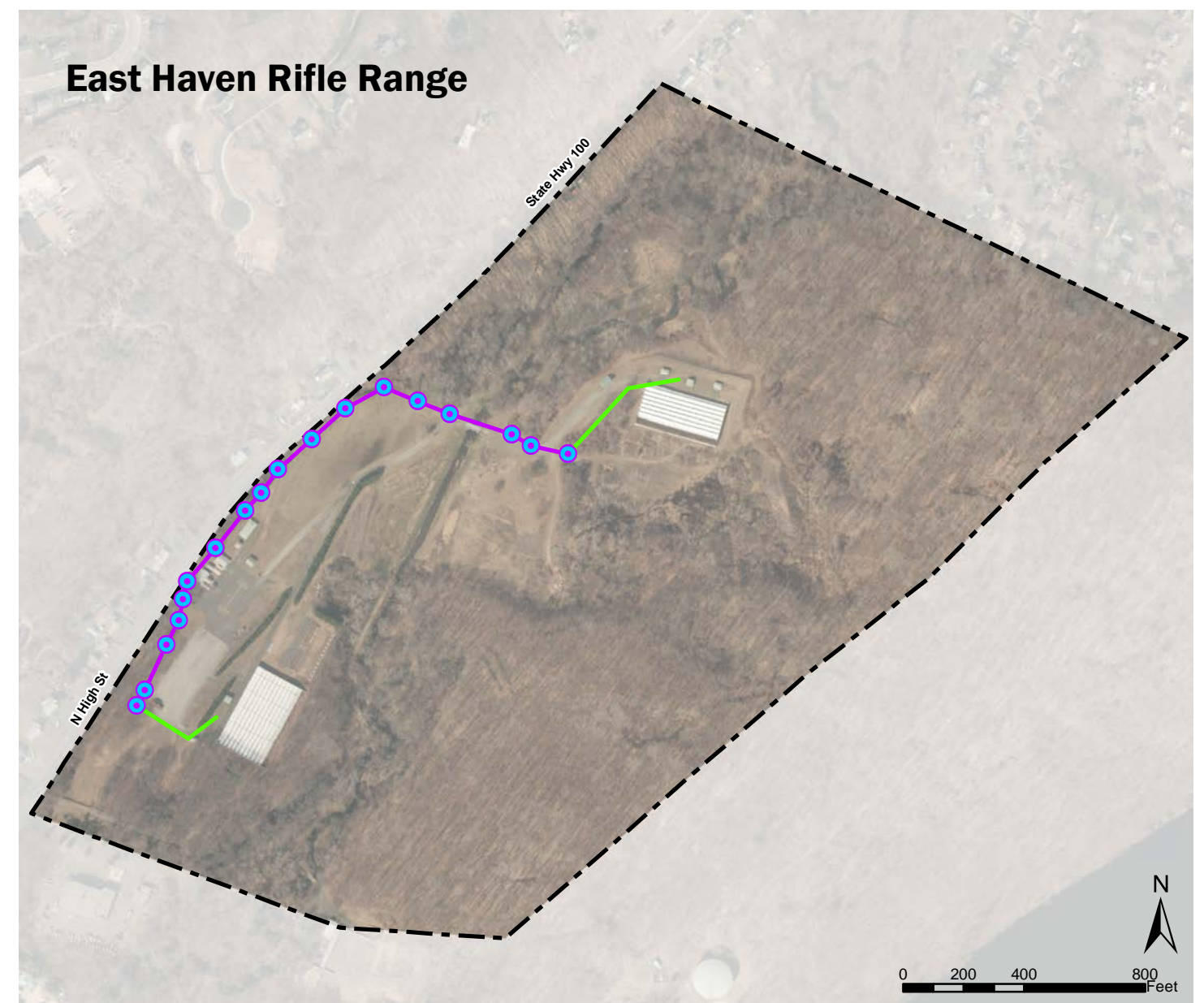
FIGURE 13: EAST HAVEN ELECTRICAL Power Pole Overhead Electrical Distribution Underground Electrical Distribution Installation Boundary
