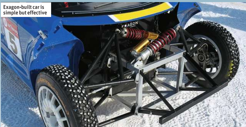
Tubular chassis carries Siemens 67Kw engine
