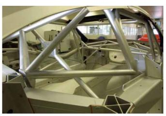
Rollcage is integrated into DBR9's bonded aluminium structure at build stage
