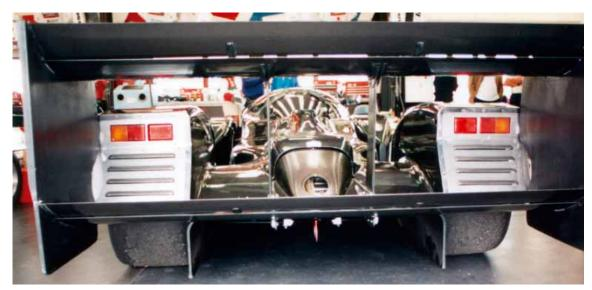
Twin-tier rear wing allowed adjustments to be made to front/ rear aerodynamic balance and also to frontal downforce
