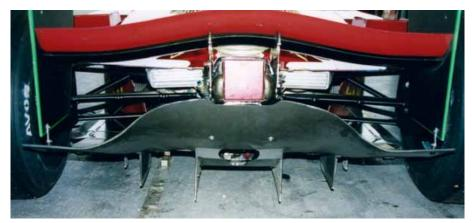
A more fundamental change at the rear on the Mansell Motorsport car is the use of a B194 rear diffuser
