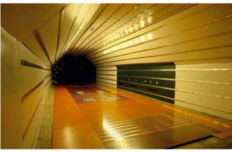
Above: internal tunnel dimensions have been honed to perfectly suit the shape of the NASCAR racecars Below: four individual rollers support unsprung weight only and spin the wheels at 130mph, while the vehicle chassis is firmly attached to four hydraulic rams. Perforations prevent boundary layer build-up
