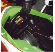
There are no hydraulic and electronic systems on Mansell car, so paddle shift has been replaced with conventional mechanical sequential shift
