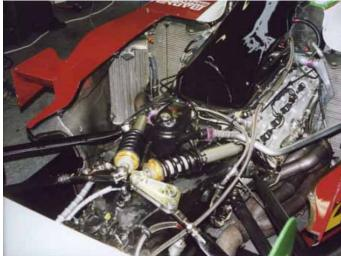
Rear suspension pickups had to be re-engineered to fit the relocated gearbox
