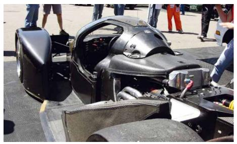
Allard. For an independent designer being paid by Originally designed to use a small block Chevy, the J2X was built with a Group C compliant Cosworth DFR
