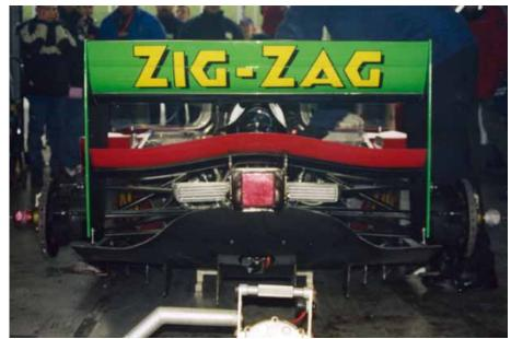
team has made, particularly on the aerodynamic side of things. But this is not about hours in a wind tunnel – it's a long time since this particular car has been near one of those – it's about where the car was when it was original designed, and where it might have been had the regulations differed. Post 1994, in the wake of the Senna tragedy, Fi cars were required to have a stepped-bottom, so fitting a flat floor to one of these cars is an obvious way to find some extra downforce.
