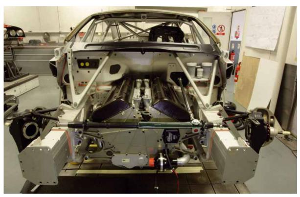
GT regulations forbid moving the bulkhead itself but the DB9's favourable engine bay layout means engines can be located further back and lower in the chassis than some of its competitors
