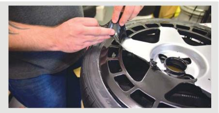
order to reveal fresh alloy. It's a popular finish seen in each corner of many modern sports cars. The downside to diamond-cutting is the fact that the exposed part of the wheel needs a specialist lacquer to protect it from harm. This makes diamond-cut finishes more delicate than paint or powdercoated surfaces. Special wheel cleaners must be used.
