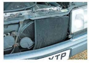
Above right: Skelton's overcooling solution is low tech... thermostat had opened and in order that K Seal shouldn't congeal around the housing, I drained the system, poured in my coppery coloured goo, added water and started the car once more. A few high-revs miles later, I seemed to have a watertight car. And one which made it back to the Fens later that evening.
