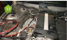
**13** Being a professional operation, TWC use a pump-type device to refill the gearbox – a lot quicker and easier than using a funnel, though the latter is fine in an environment where time isn't money. Start by measuring into the pump the exact-same amount of fluid as you know came out, not forgetting to allow a little for 'spillage' and the ATF that was soaked up by your cleaning rags etc.
