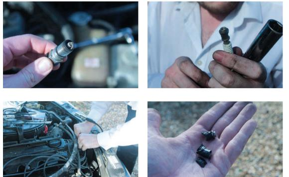
**Left:** Bits of lead had melted onto the plugs
