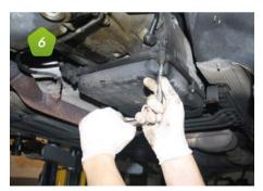
engaged as these fixings are easily mangled. Once you're down to the last couple you need to prepare for the sump to come down as the last ones are released, though if it's tight you might need a couple of mallet-taps to the side to free it.
