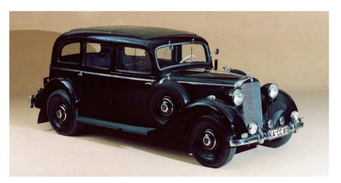
revamp in 1937. After only a year of production, the W138 chassis was replaced with the new W143 chassis, which the 260D would share with the petrol-powered 230 model. The new chassis brought new possibilities for taxi firms, making the 260D available in Landaulet form or as a fully open car. Taxi operators wanting to give their customers something more lavish to ride in could even order the 260D as a Pullman limousine.
