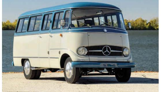
the bus has been fitted with a 2.3-litre fuel-injected M115 engine, adjustable air suspension and modern front seats for long-distance comfort.
