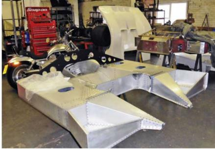
Body tub had to be completely repanelled because bonding had failed - not great when up against the clock
