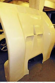
Dummy front ends produced to test original mould
